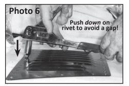
some suggestions. Try one of the pop rivets provided. Or you can pop a rivet in a piece of scrap sheet metal. Grind off the back of the pop rivet so you can extractit, with the head of the pop rivet intact. Then take a hammer and a 1/16"- diameter punch (or a nail) and knock out the rivet head from the underside. Glue pop rivet head in place in that hole in the Hood Louver panel. J-B Weld, a strong, two-part epoxy, is excellent for this. Another option is to get some longer pop rivets.
